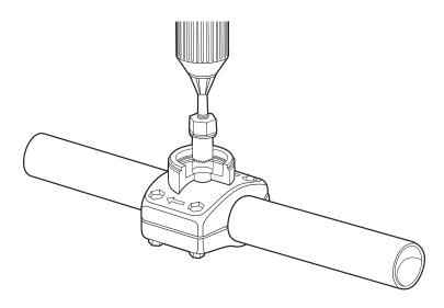
9. Insert the flow diverter into the clamp assembly and snap it into place. Snap the outer housing onto the clamp assembly.
