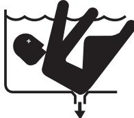
**SUCTION HAZARD.** Can cause serious injury or death. Do not use this pump for wading pools, shallow pools or spas containing bottom drains, unless the pump is connected to at least two (2) functioning suction outlets.
