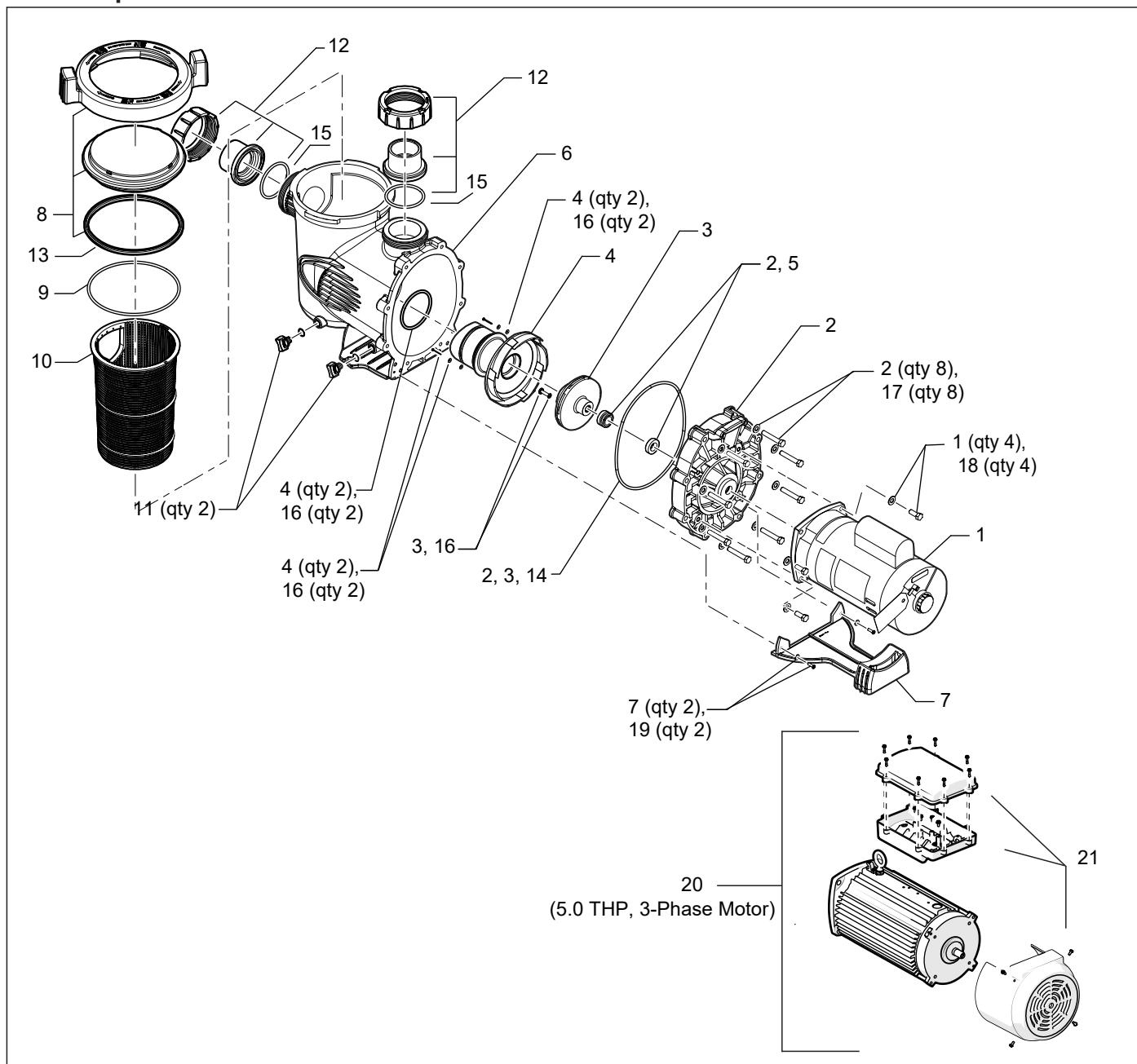
Figure 6. SHPF and SHPM Exploded View
