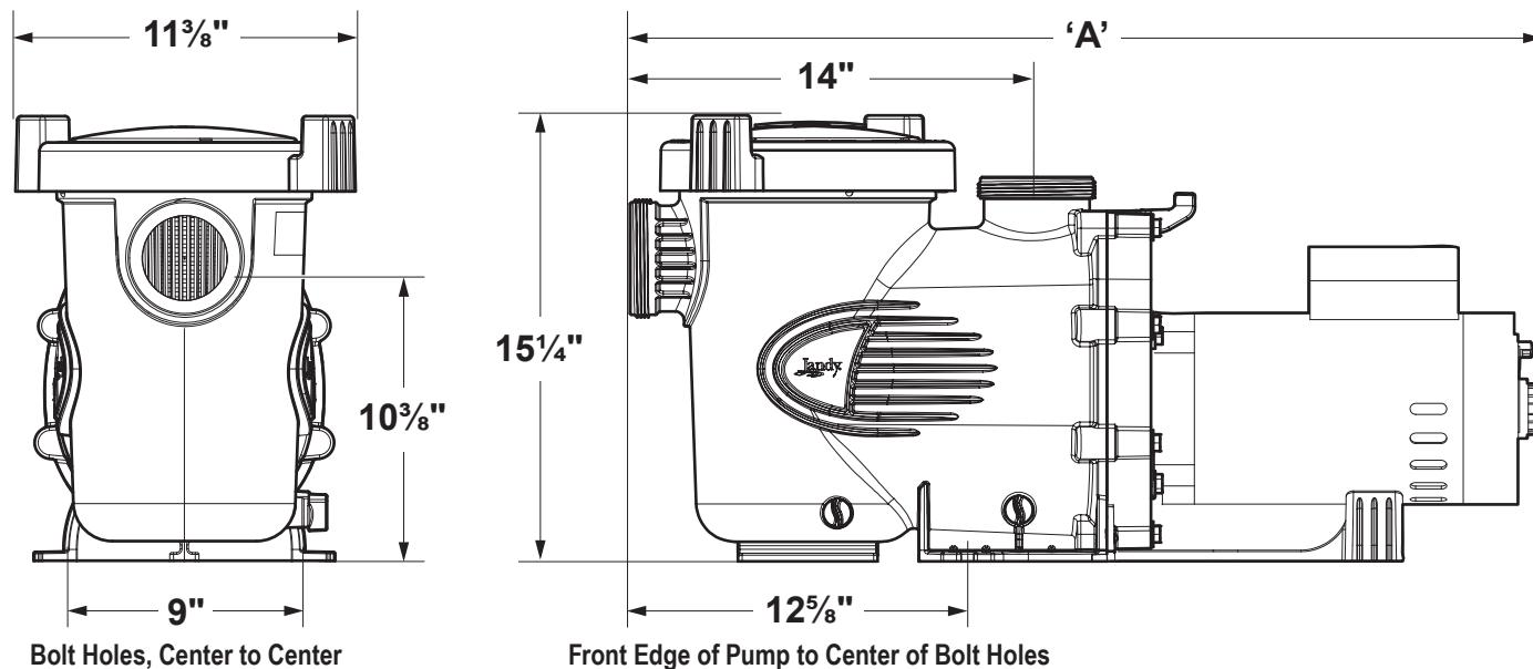
**NOTE** When installing pump, leave a minimum of two feet (2 ft) of clearance above the pump for removal of strainer basket.
