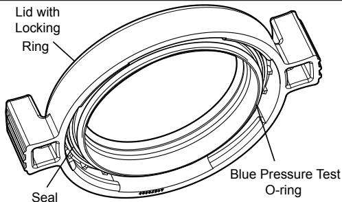
**Figure 4. Blue Pressure Test O-ring in Lid Assembly**
